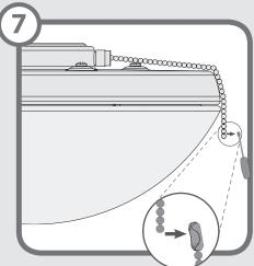
Installing the pull chain pendant Attach the pull chain pendant to the
